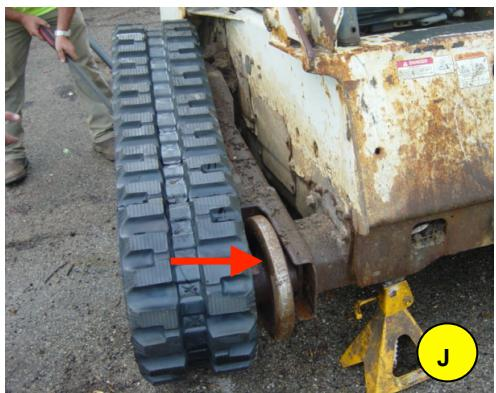
Place the inside of the new track on the front of the frame (J). This will allow you to begin using the Beaver Tail and the Armadillo together for the final stages of this process.
