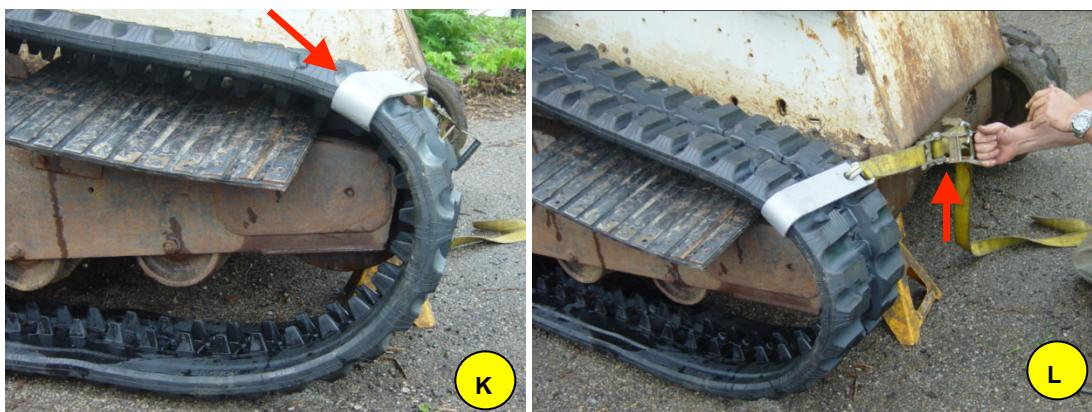
In many applications, the new track poses a serious safety problem for the installer due to the fact that they are very heavy and extremely tight. You can work for hours the old way trying to get these new tracks on, but we can do it in just minutes. By using the Armadillo to align the cogs over the front idler, it is relatively easy to pull the track in place with the Beaver Tail.
