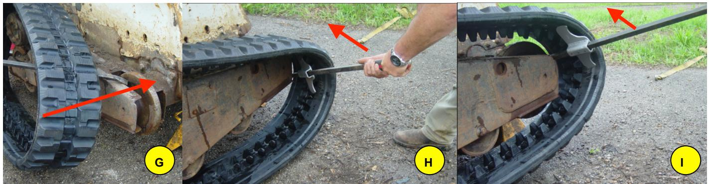
Once the rear of the new track is in place (F), use the Hammerhead to move the front of the track onto the frame (G). You will appreciate the leverage you achieve with the Power bar at this point. Use the Hammerheads wide span to leverage the track right onto the front of the frame onto the idler if possible (H,I).
