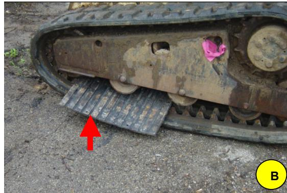
Remove the grease fitting (A). Install Armadillo mat in either the top or bottom frame (B).
