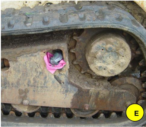
You will notice the grease coming out of the fitting (E). This is what it is suppose to do and the tension is relieved.
