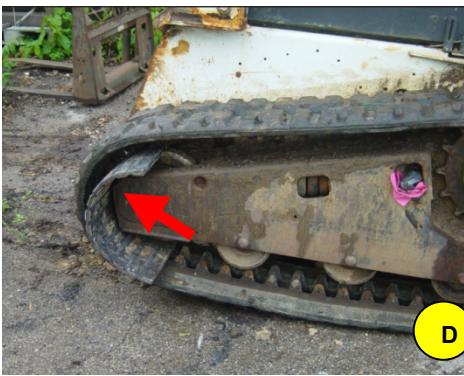
Advance the Armadillo mat to separate the cogs from the idler (C). Stop advancing the Armadillo mat at this point (D).
