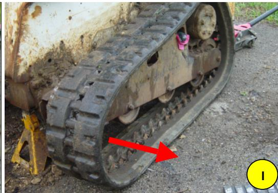
Using the side of the Hammerhead, find the optimal prying spot to begin to move the used track away from the machine (figure F & G above). Once the track is moved a couple inches, use the hook on the Hammerhead and grab the track, pulling the track away from the machine (figure H above). The track can now be removed from the machine (I).
