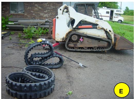
The machine and work area is now ready for the new tracks (E).
