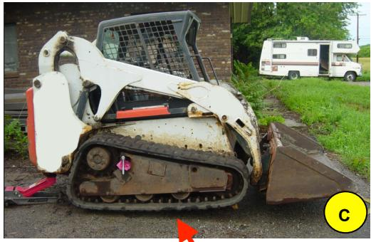
The machine has 2 supports placed securely under the front and back of the machine on the same side as the track that you will be working on. Notice the track is only 3"- 4" off the ground (C). The opposite side track is firmly on the ground. Always make sure you're the machine is properly supported.
